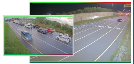
A key advantage of WWVDS is the coordinated response it enables. When an alert is triggered, Traffic Management Center (TMC) operators quickly manage the situation, activating response plans that include warnings on DMS boards and coordinating with the Florida Highway Patrol (FHP). "The operators would be able to search the screenshots... to determine if it's a true wrong-way driver that requires activation," explained Mikol. This quick decision-making is essential in preventing collisions.
