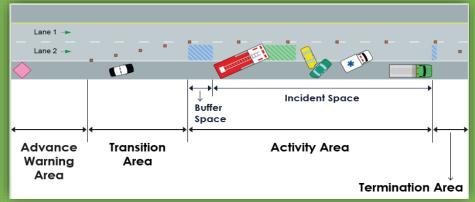
Management area. Protects emergency responders working at the end of the Incident Space. Includes the downstream buffer space and taper. Remember drivers will likely be frustrated from being stuck in traffic and may quickly accelerate.
