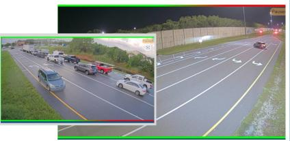
A key advantage of WWVDS is the coordinated response it enables. When an alert is triggered, Traffic Management Center (TMC) operators quickly manage the situation, activating response plans that include warnings on DMS boards and coordinating with the Florida Highway Patrol (FHP). "The operators would be able to search the screenshots... to determine if it's a true wrong-way driver that requires activation," explained Mikol. This quick decision-making is essential in preventing collisions.
