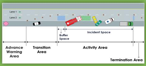
Management area. Protects emergency responders working at the end of the Incident Space. Includes the downstream buffer space and taper. Remember drivers will likely be frustrated from being stuck in traffic and may quickly accelerate.
